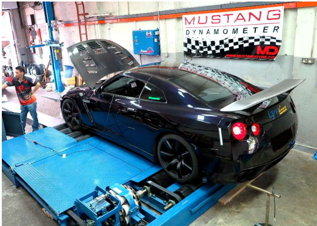
Figure 3 Mustang 4WD dyo with PAU and belt covers removed
